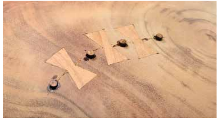
The drilled holes with the huini glued in place ready for cleaning up and sanding
