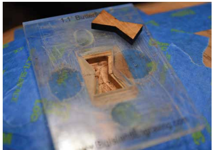
Here is the fill depth recess and the corresponding pewa to be inset
