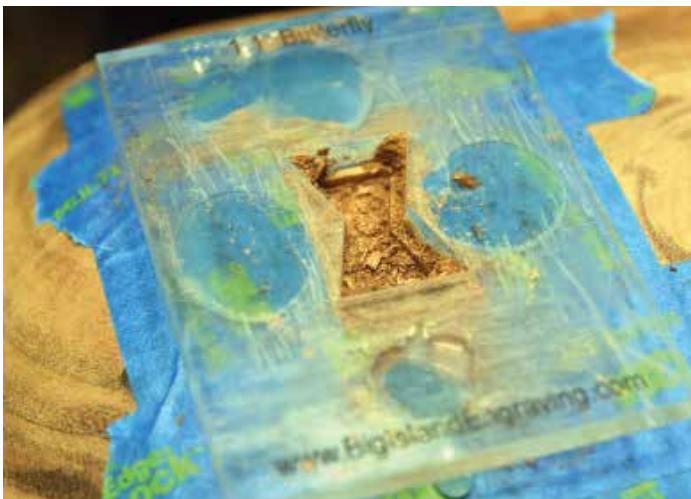
Stop regularly and clear out the debris
