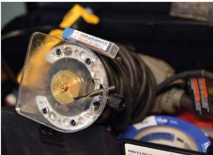
The picture shows the router with guide bush and bit attached and a spare router bit to show what is being used to cut the wood
