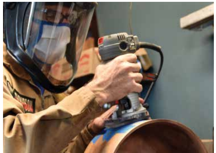
Wearing appropriate PPE and RPE and keeping the router firmly against the template, make gentle cuts, incrementally deeper until the required depth is achieved
